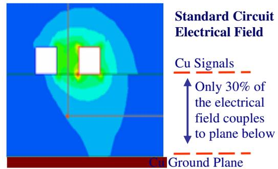
Figure 5 – Electrical field and typical ground plane below.
