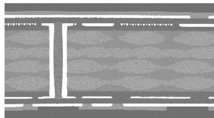
Table and Figure 2 – Substrate with laser formed circuits.
