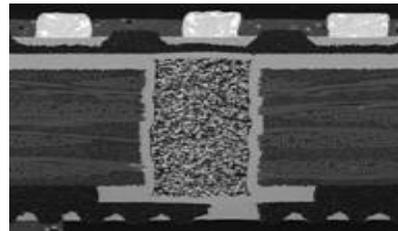
Table and Figure 1 – Substrate with laser formed circuits.
