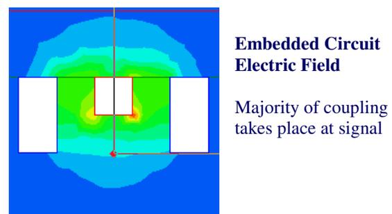
Figure 6 – Embedded circuit and electrical field.
