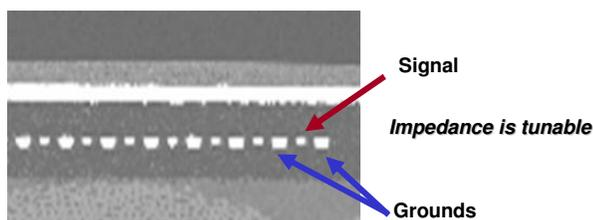
Figure 4 – Coplanar ground embedded circuits.
