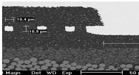
Table and Figure 3 – Substrate with laser formed circuits.
