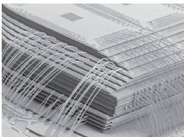
3-dimensional (3D) packaging technologies exploit the third or Z-height dimension to provide a volumetric packaging solution for higher integration and performance. 3D packaging has become critical to integrating the multi-media features consumers
